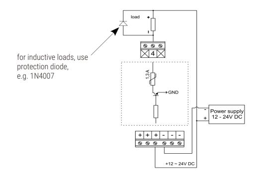
Inside the device at each outputs is protective thermistor PTC 1.3A, which one in case of breakdown (short circuit, overload), during the increase of resistance the temperature will rise the thermistor will disconnect.
