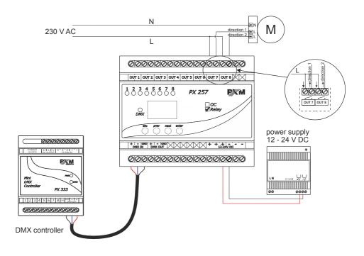
**NOTE:** If you want to connect an electric motor to the device, it has to be connected to paired outputs (e.g. output 1 - 2 / OUT1 - OUT2). If connected to unpaired outputs, may damage the motor or device PX257.
