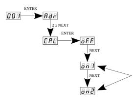
once this feature is enabled, you can modify delay time (adjustable in the range of 0.1 to 5s) between one of the outputs in a pair being switched off and the other output being enabled An example of connecting an electric motor with two directions of rotation to device PX257
