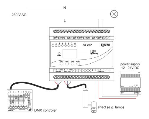
c) version PX257–RE – at high load, use a contractor with connected external power supply to receivers
